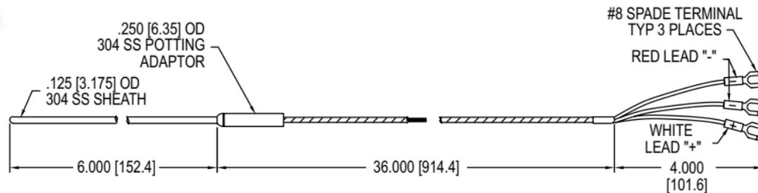
Precision **Series RTD Resistance Temperature Detector** offers excellent accuracy and stability over a wide temperature range. Industry standard 3-wire 100  $\Omega$  (DIN) probes are available in 6" (15 cm), 12" (30.5 cm), or 18" (46 cm) sheath lengths with 30" (76 cm) extension cable and spade lug terminals.
