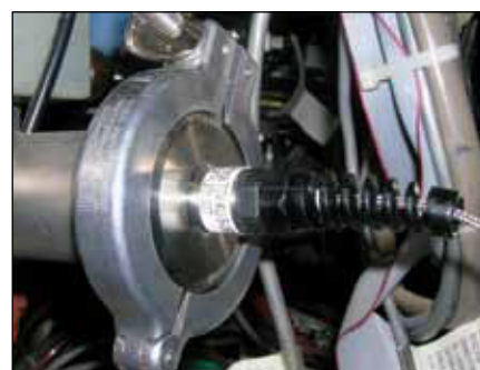
TCV probe shown installed using customer supplied clamp and O-ring.
