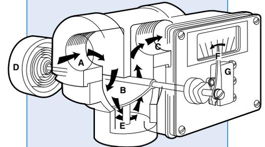
Fluid enters at **A**, passes around the semi-circular vane **B**, exits at outlet **C**. The vane resists the flow because of the spring **D**. The further the vane is pushed the larger the passageway **E** becomes. This minimizes the pressure drop. The vane shaft turns to operate the pointer **F** and remote signal devices such as the switch **G**.
