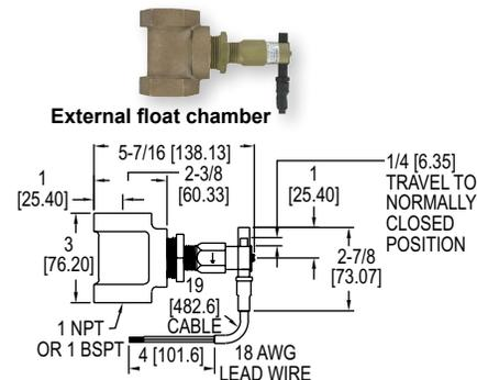
The **Series L10 Flotect® Mini-Size Float Switch** is a series of economical, compact liquid level floats. It is offered in brass or 303 SS bodies and external tees as well as polypropylene or 304 SS floats with 1" NPT male threads, for direct side mounting through a half coupling, or with factory installed tee for external mounting. This series can be used in liquids with specific gravities as low as 0.5.
