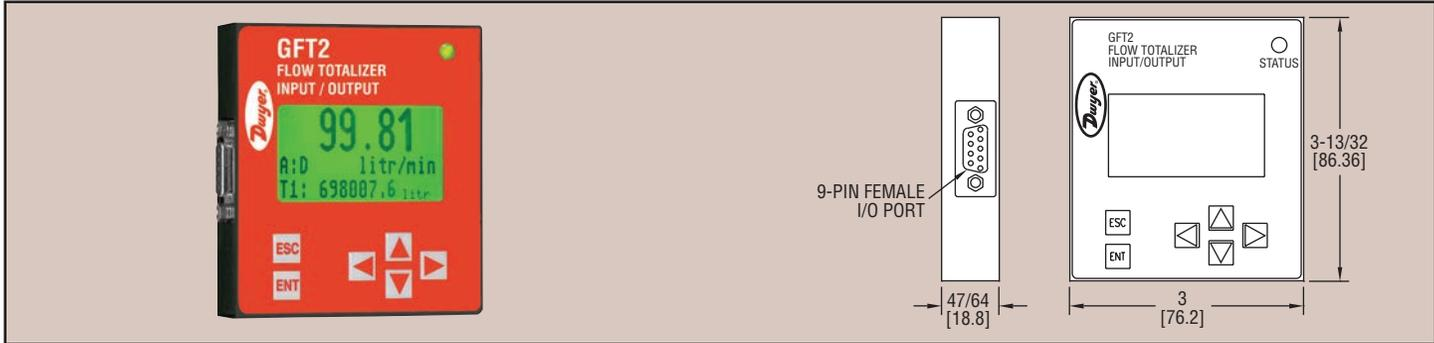
The Series GFT2 Flow Totalizer is a microcontroller driven device designed to linearize the flow meter and controller flow curve plus display the instantaneous flow rate, total, and accumulated total. The totalizer is intended to be used with analog flow meters and controllers with analog 0 to 5 VDC, 0 to 10 VDC, or 4 to 20 mA interface. RS-232 or RS-485 digital interface is available.
