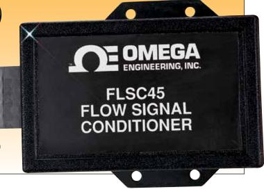
selectable output across a dedicated flow range. The high-performance electronics will accept a low-level magnetic pickup signal from a paddlewheel or turbine meter without amplification. The industry-standard output interfaces directly with OMEGA's iSeries meters and controllers. The FLSC-45 features a plastic enclosure with a built-in mounting plate for wall mounting.
