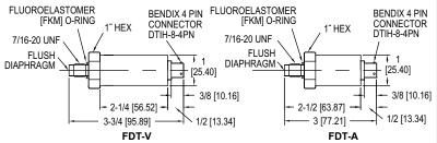
The **Series FDT Flush Diaphragm Transmitter** is designed for highly cyclical conditions. Flush sensor feature prevents any potential inaccuracies due to build-up or blockage which is a typical problem found in most non-flush transmitter sensors.
