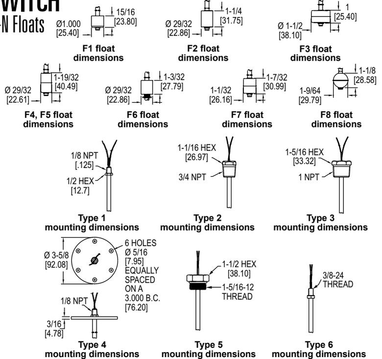
The **Series F7-MM Miniature Multi-Station Level Switch** provides a customized level switch to meet application requirements in a miniature size. Control up to five different level points across a maximum length of 48" (121 cm). Stems and mounting fixtures are available in 316 SS or brass.
