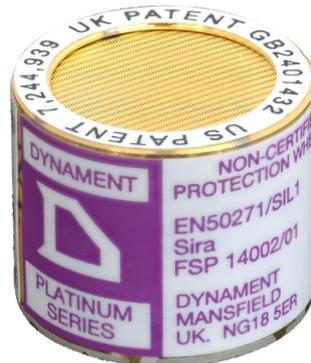
The Platinum series sensors contain all the necessary optics, electronics and firmware to provide a linearized, temperature-compensated output. Within the Platinum series are low-power options and dual-gas, high resolution methane / carbon dioxide sensor that provides the capability to simultaneously monitor methane and carbon dioxide in a single sensor package, consuming the power of a single infrared sensor.
