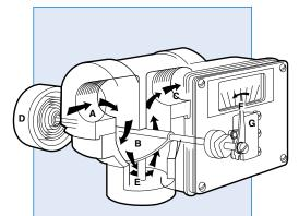
Fluid enters at **A**, passes around the semi-circular vane **B**, exits at outlet **C**. The vane resists the flow because of the spring **D**. The further the vane is pushed the larger the passageway **E** becomes. This minimizes the pressure drop. The vane shaft turns to operate the pointer **F** and remote signal devices such as the switch **G**.
