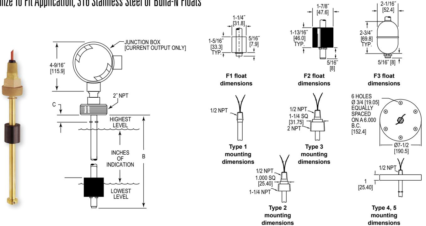
The **Series CLT Continuous Level Transmitter** provides up to the minute tank level monitoring with a customized level transmitter. Transmitters can be configured for 4-20 mA or proportional voltage output, 316 stainless steel or Buna-N stem and floats, and lengths up to 72" (183 cm).
