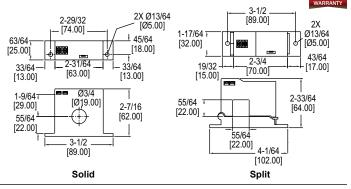
The Series CCT40/50 Current Transformers are a low cost alternative for measuring power and monitoring the operation of fans, pumps, or other equipment. For use on existing installations, split core models can be installed without disconnecting cables. Each model offers three jumper selectable ranges and a choice of three different outputs.
