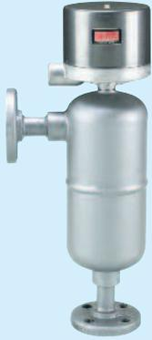
Series 253 has one vertical and one horizontal flanged connection (1" RF forged steel - ANSI specifications). Flange centerline 14" (356 mm). Other centerlines available.
