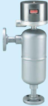
Series 1263 has one vertical and one horizontal flanged connection (1" RF forged steel - ANSI specifications). Flange centerline 14" (356 mm). Other centerlines available.
