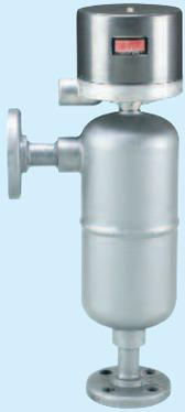
Series 1253 has one vertical and one horizontal flanged connection (1" RF forged steel – ANSI specifications). Flange centerline 14" (356 mm). Other centerlines available.
