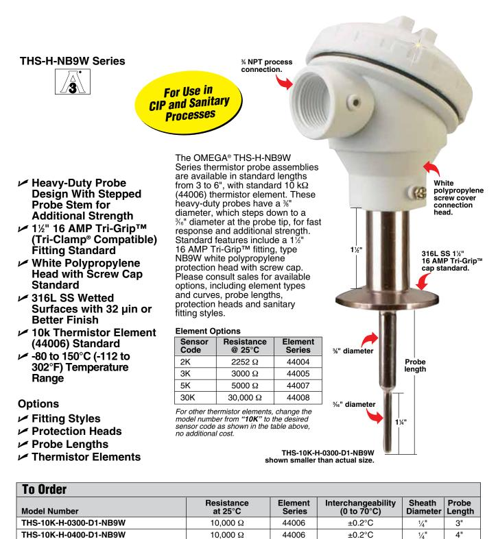
For lengths longer than 6", change **"0600"** in model number to the required length (eg, 12" = 1200,  $9'_4" = 0925$ ) for an additional cost. To order with **NB15** large 316 SS head, change model number suffix from **"-NB9W"** to **"-NB15"** for an additional cost. **Ordering Example: THS-10K-H-0400-D1-NB9W**, 10,000  $\Omega$  thermistor sensor,  $1'_2"$  16 A Tri-Grip<sup>TM</sup> fitting, 4" length, heavy duty probe, NB9W white polypropylene screw cap protection head.
