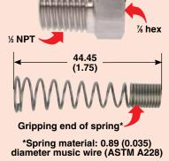
Spring loaded fitting for use with SLF-12-12-14 0.25" ½ NPT connection heads
