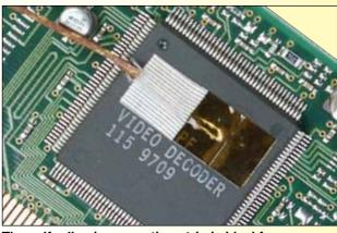
The self-adhesive mounting strip is ideal for "targeted" placement of the sensor element. Once the element is in place, it can be used "as is", for applications such as electronic component temperature monitoring during board fabrication. It can also be cemented in place using OMEGABOND® for higher temperatures.
