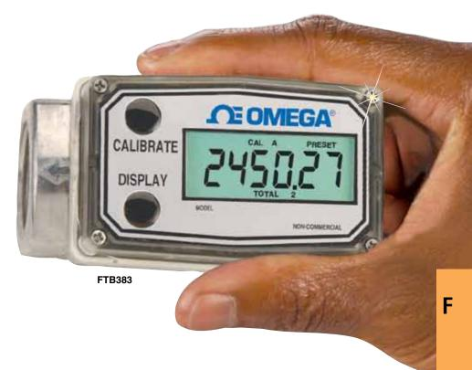
FTB380 Series turbine meters with microprocessor-based electronics offers a durable, compact, highprecision fuel measurement device, with total and rate indication. Information is clearly displayed on a large 6-digit liquid crystal display with only 2-point floating decimal for totals from 0.01 to 999,999. All operations are easily performed with only 2 buttons.
