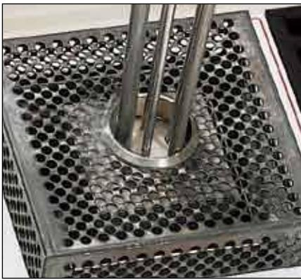
CL950 multi-well accepts up to 5 probes at one time and comes standard with 1/16, 1/8, 3/16 and two 1/4" diameter holes.
