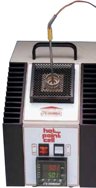
CL900-110 hot point® dry block calibrator with DSS-460-K benchtop thermometer (see omega.com), calibrating a single thermocouple probe, shown smaller than actual size.
