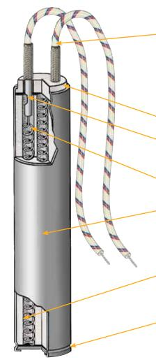
The standard termination for low-density cartridge heaters is Type F, consisting of 254 mm (10") internally connected flexible lead wires with high temperature insulation, UL approved for 300 or 600V service and temperature rated to 250°C (482°F).
