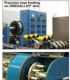
Horizontal wrapping of alumina fiber insulated wire.
