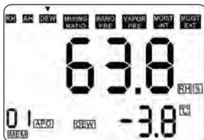
In Dew point measurement mode, **DEW** will appear at the left of the secondary readout to remind you that the value shown reflects the dew point temperature, rather than the ambient temperature.
