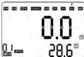
To obtain accurate readings in **MOIST INT** mode, you should reset the readout to 0.0% each time you re-enter that mode from another mode.
