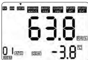
**Holding readings.** Briefly pressing the **ON/OFF HOLD** button freezes both the primary and secondary readouts. **HOLD** will appear on the display to remind you that the readouts are frozen.
