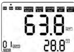
The RH650 can measure and display the value of eight different moisture-related parameters. When the meter is in measurement mode, you select a parameter by pressing either the **UP>** and **<DN** buttons to move the ▼ pointer on the top line of the LCD directly above it. For example, the following is the display for RH measurement mode—the operating mode that the meter enters by default when it is powered on.
