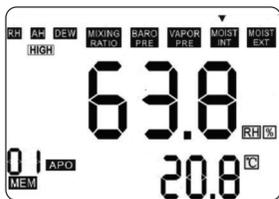
To enter Alarm set mode, press the **MAX/MIN** and **UNIT** buttons at the same time while in **RH**, **MOIST INT** or **MOIST EXT** mode. Doing so will display the current value of the selected parameter's high setpoint and cause the word **HIGH** to appear near the upper left of the display, as shown on the left.
