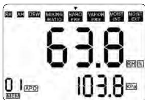
As the figure on the left shows, moving the ▼ pointer four positions to the right (by pressing the **UP>** button four times) switches the meter to operate in Ambient pressure mode.
