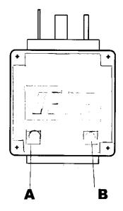
To make settings: Loosen the four Phillips screws on the display and remove the cover. The PM1000 uses a display menu, controlled by the 2 programming buttons, to assist when editing display settings and options.
