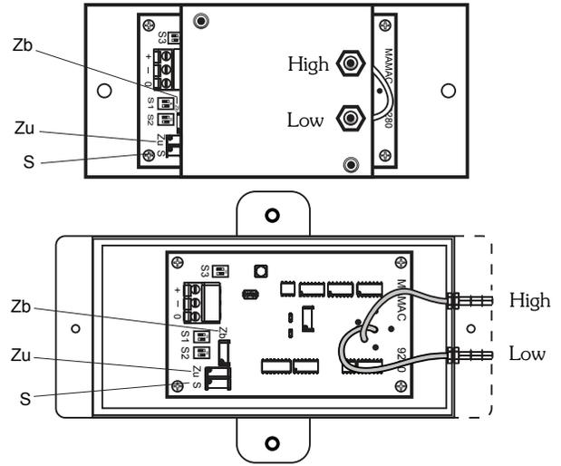
PX274/275/277/278 pressure transducers with 4-20 mA output are powered with a 12-40 VDC supply.
