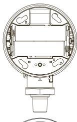
For reattachment of cover, align the 'unlock' icon with the arrow, push cover straight in then turn clockwise until the arrow is in alignment with the 'Lock' icon.
