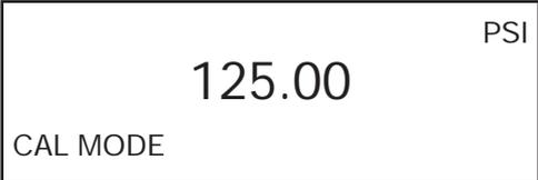
Use the Pressure Standard to output 125.00 psi (25%). After the output has stabilized, press the ENTER key to continue. As the unit takes readings, the screen will show -----. When the readings are complete the screen should look as shown below.
