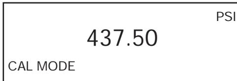
Use the Pressure Standard to output 437.50 psi (87.5%). After the output has stabilized, press the ENTER key to continue. As the unit takes readings, the screen will show -----. When the readings are complete the screen should look as shown below.
