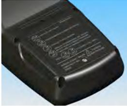
Remove the two screws on either side of the battery cover by turning them counterclockwise until the fully disengaged from the manometer base. Lift the cover from the back of the unit.
