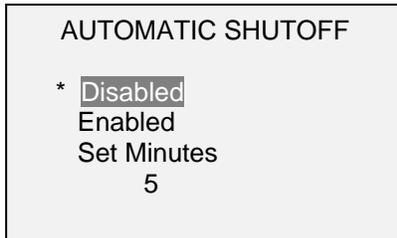
Select **Disabled** to disable automatic shutoff. Select **Enabled** to enable it. The length of time of inactivity is programmed in minutes via the **Set Minutes** parameter. Available settings: 5-30, in 5 minute increments.
