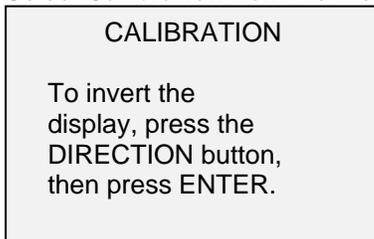
2. Press **DIRECTION** to invert the display, if desired. **ENTER** to continue. The display will appear as follows:
