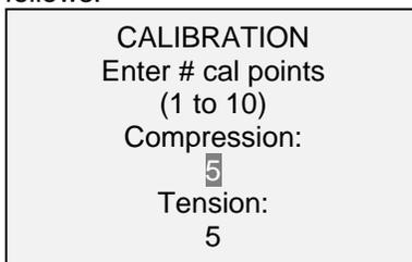
The gauge can be calibrated at up to 10 points in each direction. Enter the number of calibration points for each direction (compression and tension). At least one point must be selected for each direction.
