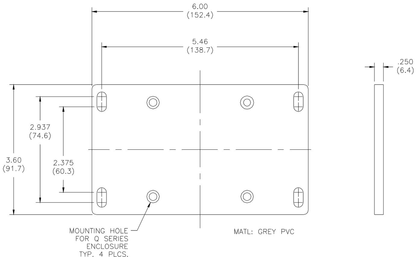
**Figure 2-3 Wall or Pipe mount Bracket**
