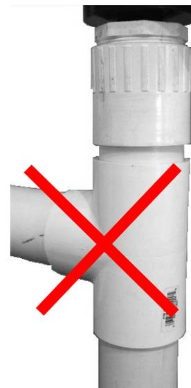
Avoid the use of a tee within the stand pipe. A tee can create false signals which will interfere with the sensor's performance.
