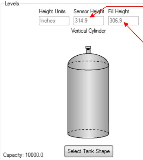
**Sensor Height:** Distance from the bottom of the tank to the bottom of the transducer.
