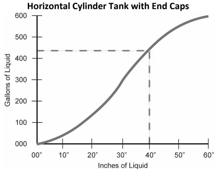
In the above illustration, 1" of liquid does not equal 10 gallons. The 10" at the bottom represents a rise of 62.8 gallons where the change between 10" and 20" represents an increase of 109.6 gallons.
