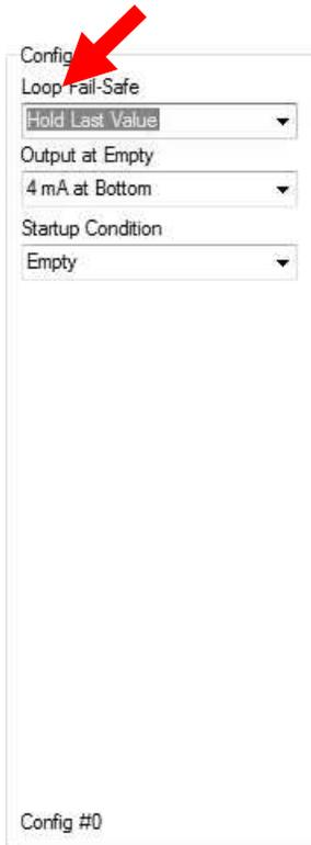
The screenshot shows a configuration window titled 'Config #0'. It contains three dropdown menus: 'Loop Fail-Safe' (set to 'Hold Last Value'), 'Output at Empty' (set to '4 mA at Bottom'), and 'Startup Condition' (set to 'Empty'). A red arrow points to the 'Loop Fail-Safe' dropdown menu.
