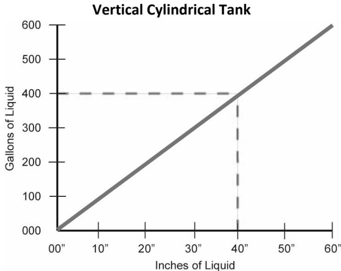
In the above illustration, 10" of liquid will always be equal to 100 gallons of liquid (1" = 10 gallons).
