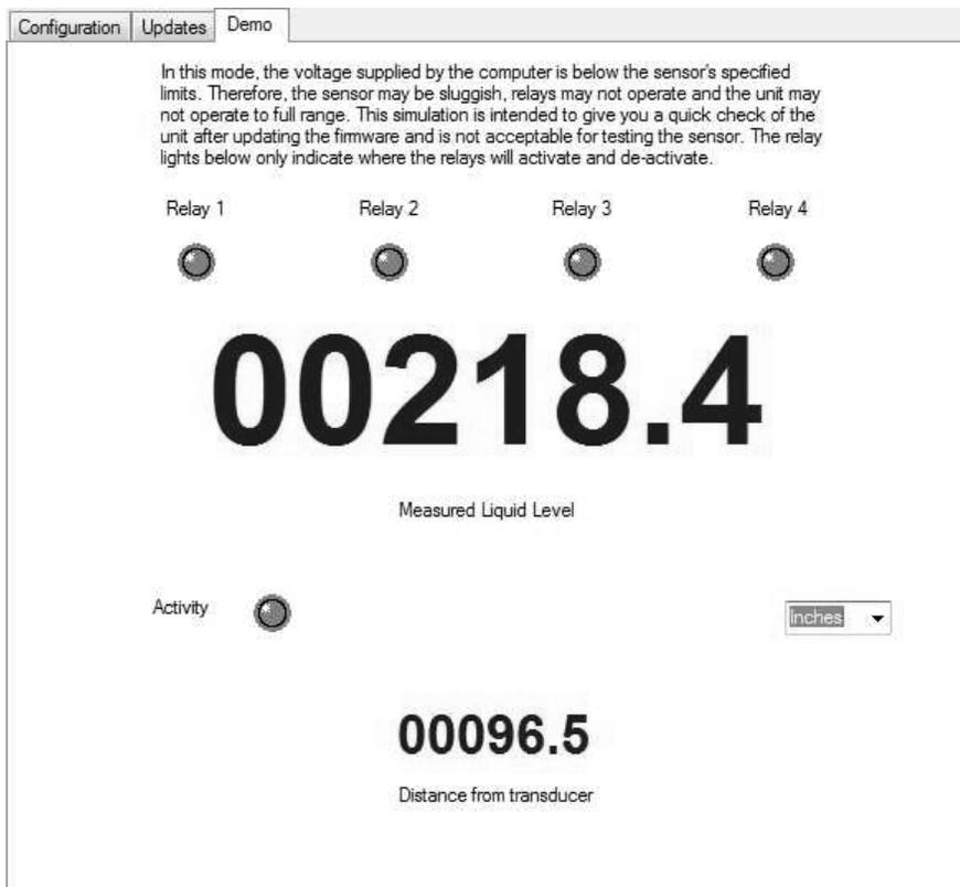
The demo page is a simulation, useful for verifying the configuration. There is not enough power going to the unit to power the relays in the Demo mode. The larger numbers represent the liquid level while the smaller numbers show the distance from the transducer to the surface.
