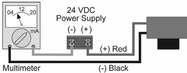
1. Connect a multimeter in series with the black wire to read the current output.
