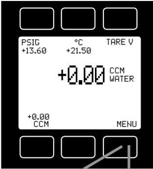
The **Main** display shows, temperature and volume flow. Line pressure will be also be displayed if the meter was order with this option.
