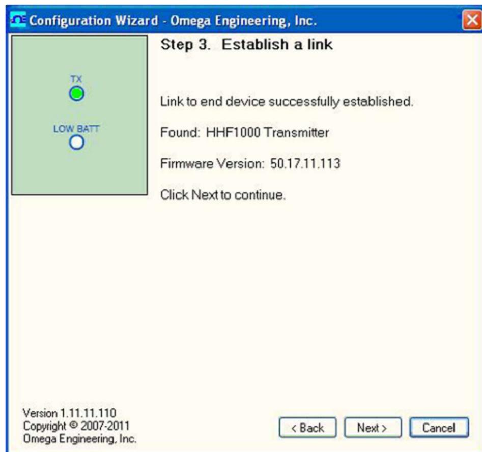
Figure 5-4. Establishing Communication With HHF1000 Screen
