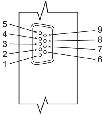
**FIGURE 2.a - 9-PIN “D” CONNECTOR PINOUTS FOR FMA1700A/1800A TRANSDUCER**
