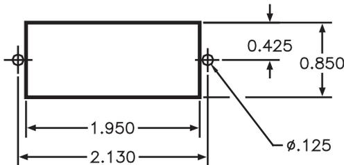
**FIGURE 2.b - CUTOUT DIMENSIONS FOR LCD PANEL MOUNTING**
