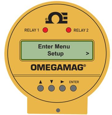
Use the keypad to navigate through each setting.
