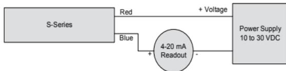
Note: 4-20 mA products are designed to operate with a maximum loop resistance of 600  $\Omega$ .
