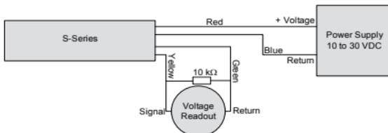
Note: to achieve calibrated accuracy the load must be 10 k $\Omega$  between Yellow and Green,
