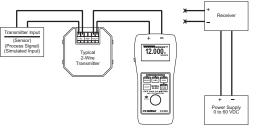
The CL532 sources 0.000-24.000 volts. This is useful for powering transmitters and receiver equipment. Use the EZ-DialTM Knob and EZ-CheckTM Switch to adjust output voltage. The display flashes "LOW  $\Omega$ " when the output is overloaded.
