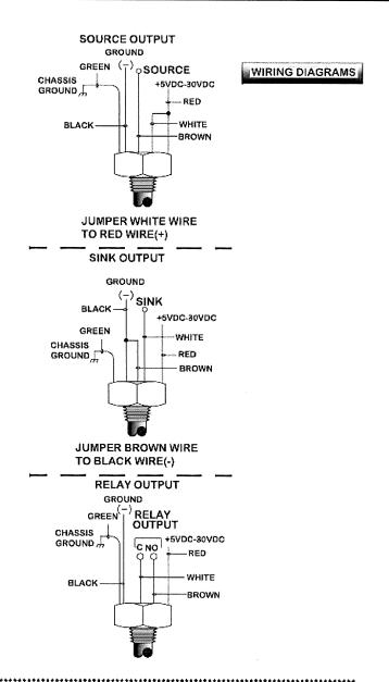
For Ultrasonic Point Level Switches
