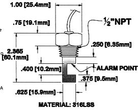
For Ultrasonic Point Level Switches
