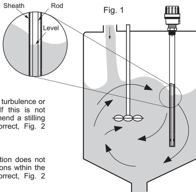
The tank must be free from turbulence or vortices throughout use. If this is not possible we highly recommend a stilling well or sheath. (Fig. 1 correct, Fig. 2 incorrect)
