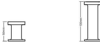
Extended necks for medium temperature (up to 120°C) and high temperature (up to 150°C)
