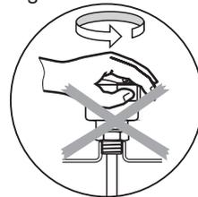
When tightening the sensor, use only use the 316S.S. hexagon fitting to achieve a seal, do not twist with the body of the sensor. (Fig. 3)
