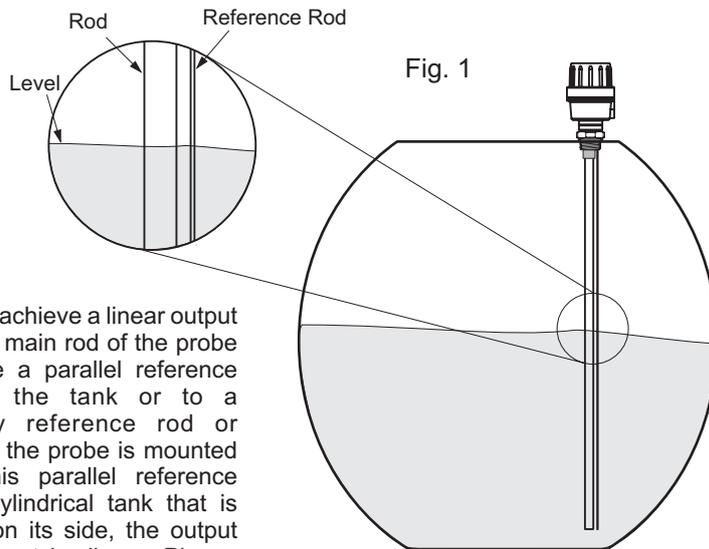
In order to achieve a linear output signal, the main rod of the probe must have a parallel reference either to the tank or to a secondary reference rod or sheath. If the probe is mounted without this parallel reference within a cylindrical tank that is mounted on its side, the output signal will not be linear. Please consult one of our applications engineers if you have further questions. (Fig.1 correct Fig. 2 incorrect)
