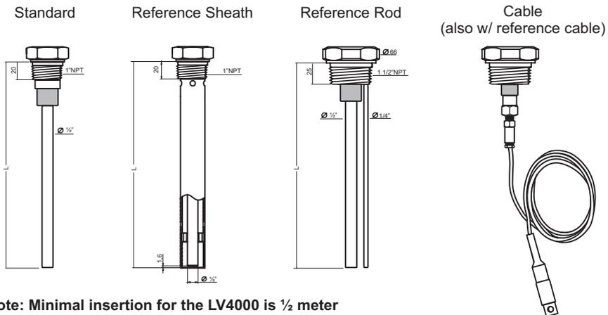
Note: Minimal insertion for the LV4000 is 1/2 meter
