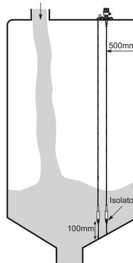
When installing the LV4000 with cable and reference be sure that they are well connected to the bottom of the tank and that it has no slack. (Fig. 1 correct Fig. 2 Incorrect)
