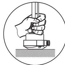
Care should be taken when handling and installing probes with coated rods to avoid scratching them. Scratching the coating could interfere with the probe performance.
