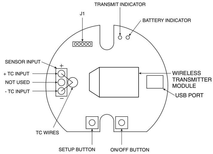
Figure 3-1. Main Transmitter Board
