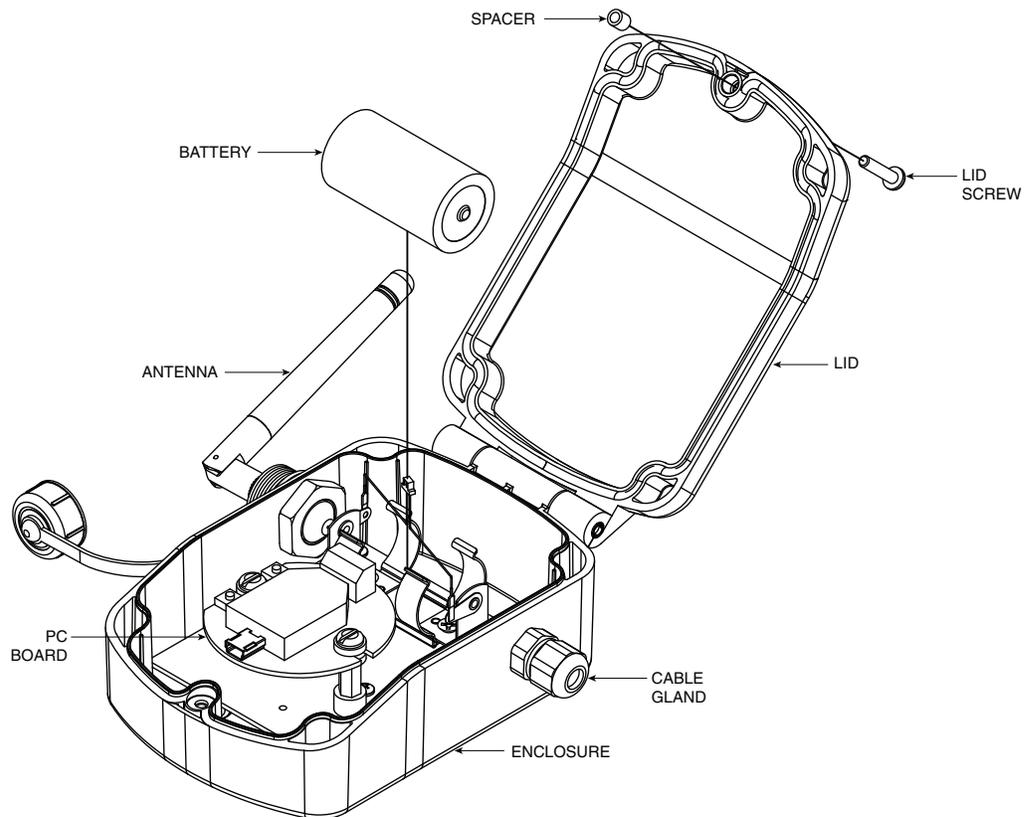
Figure 5-13. Battery Replacement
