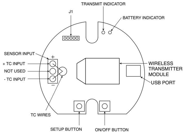
Figure 5-14. Input Connections for Cable Gland Connector
