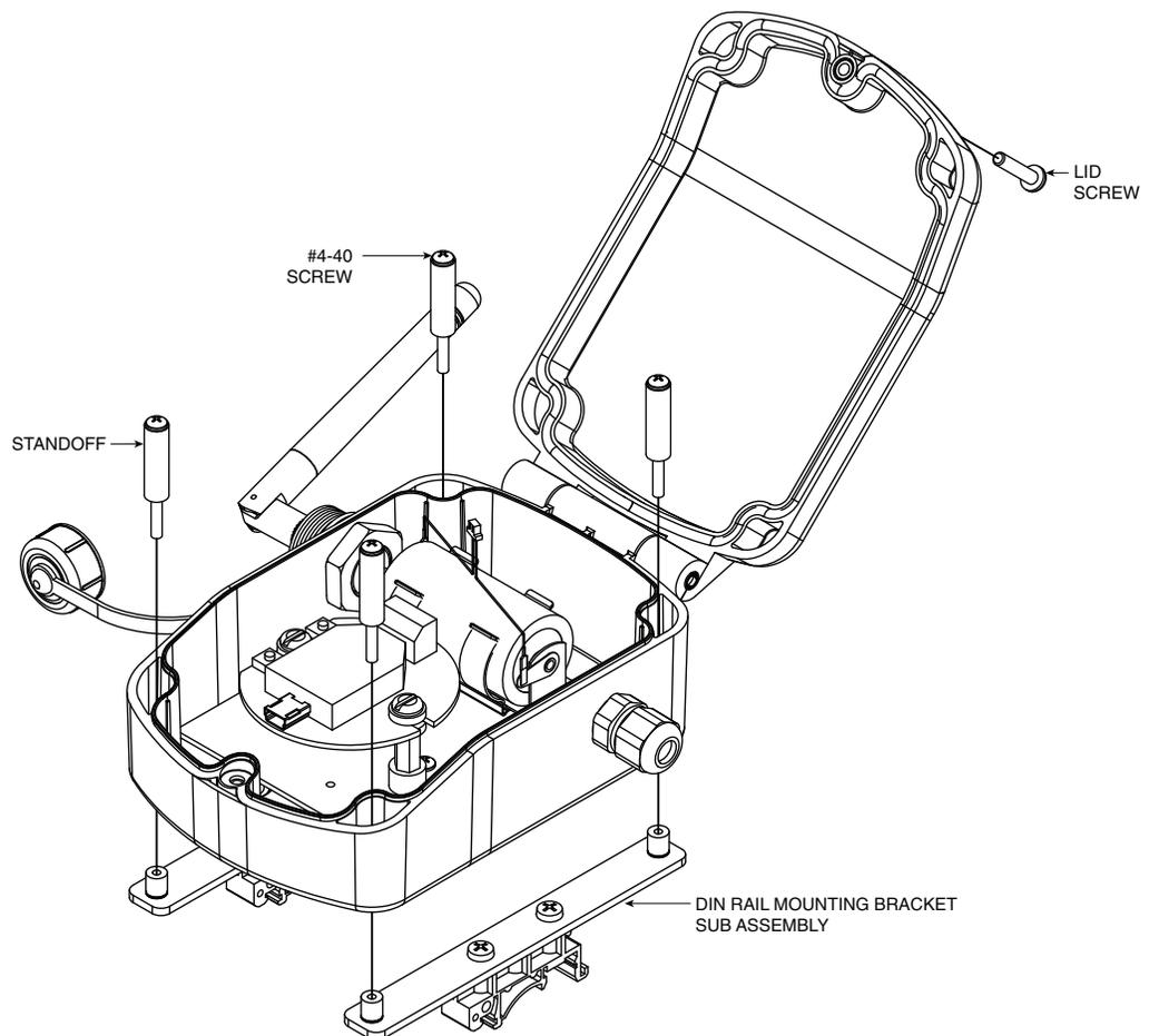
Figure. 5-12. DIN Rail Mounting Bracket Installation
