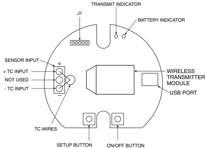
Figure 5-2. Main Transmitter Board
