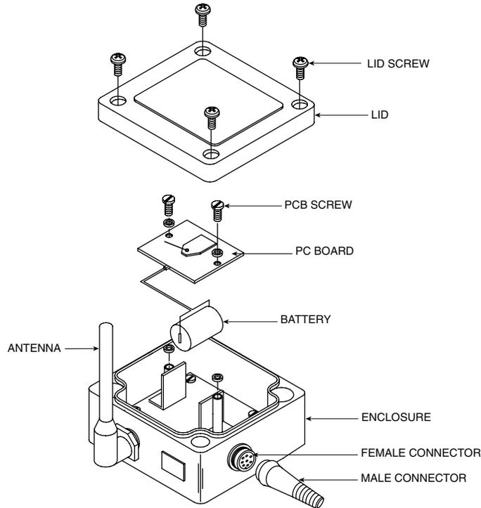
Figure 5-12. Battery Replacement
