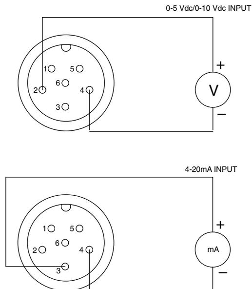
Figure 5-14. Input Connections
