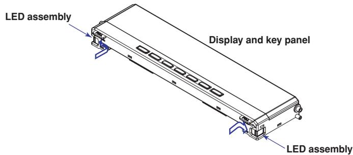
4. Remove the LED assembly from the connector of the flexible printed circuit board.
