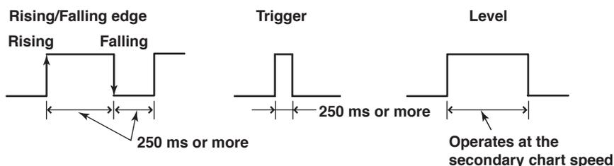
For contact inputs, the remote signal rises when the contact switches from open to closed and falls when the contact switches from closed to open. For open collector signals, the remote signal rises when the collector signal (voltage level of the remote control terminal) goes from high to low and falls when the collector signal goes low to high.
