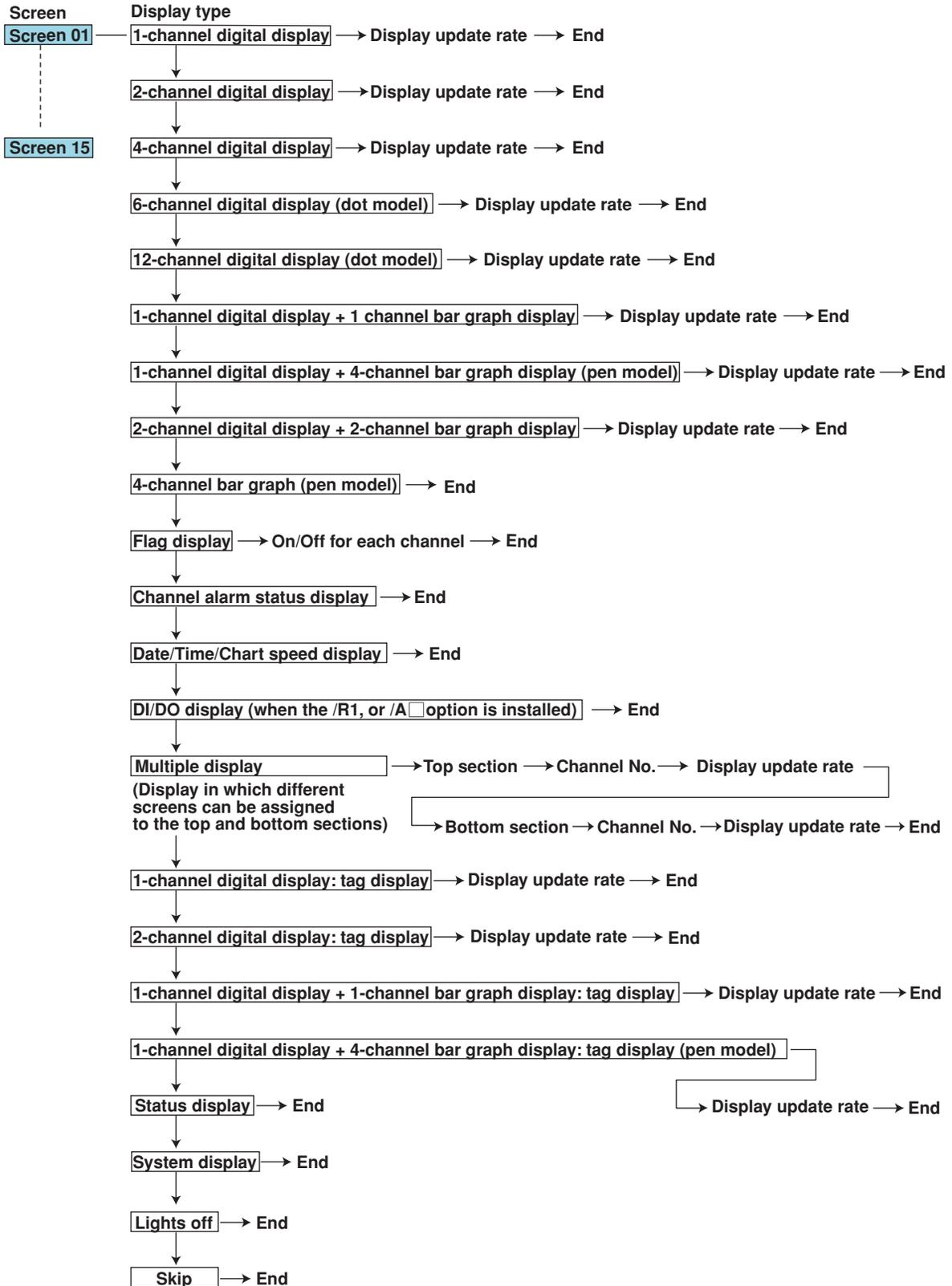
The display update rate corresponds to "Interval" in the setup menu. It is the time interval at which the displayed channel is switched.
