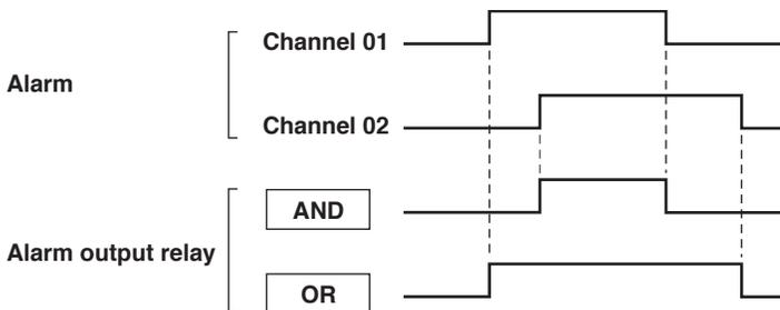
The alarm output relays assigned to AND operation are specified as follows: “I01 (first relay) to Ixx (where xx is the relay number).”
