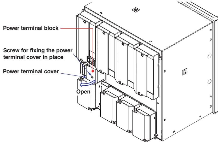
2. Wire the power cord and the protective ground cord to the power supply terminals.
