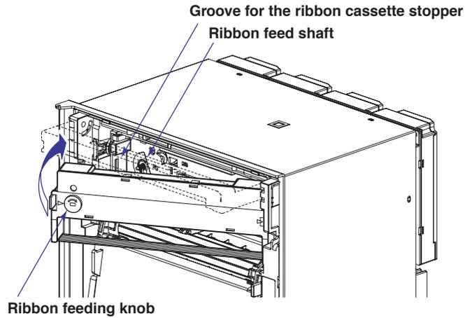
8. Turn the ribbon feeding knob in the direction of the arrow a half turn or more to check that the ribbon is feeding properly. If the ribbon is loose, turn the knob in the direction of the arrow to tighten it.
