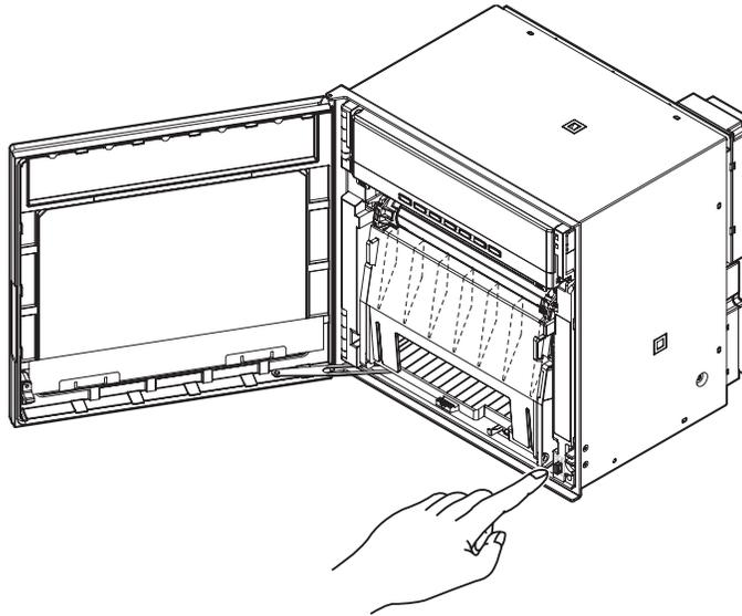
When the power switch is turned ON, a self-diagnosis program runs for a few seconds, and the recorder is ready for operation.
