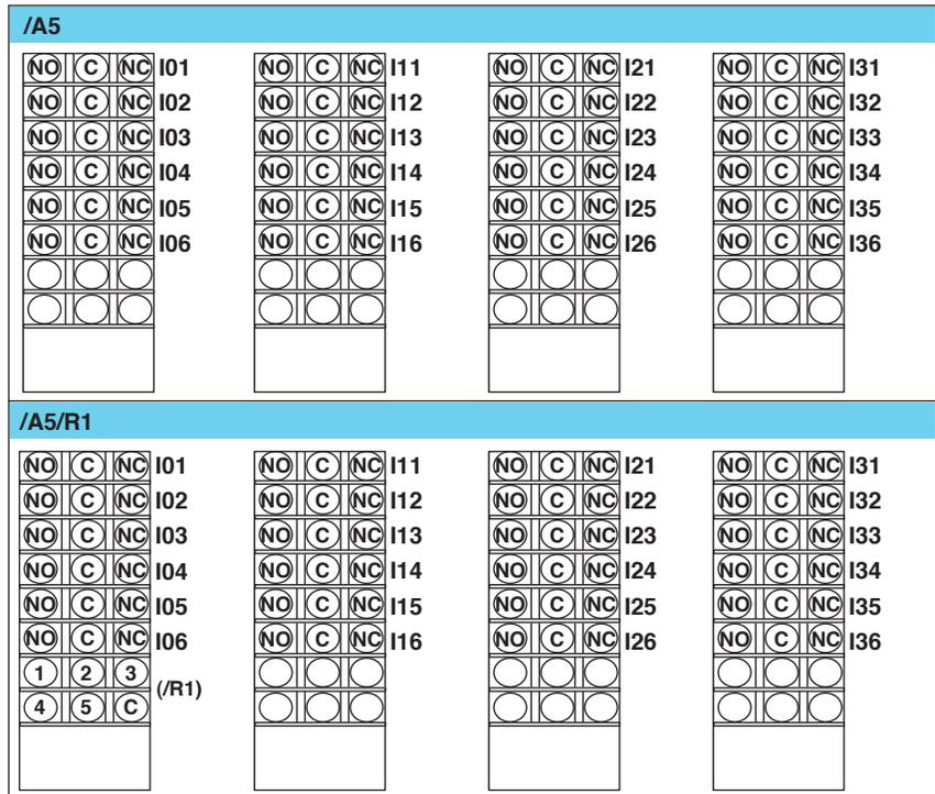
**Alarm Output Relay Terminals and FAIL/Chart End Output Relay Terminals**
