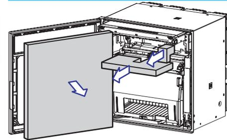
Return the display and key panel section to its original position by pressing the section downward.
