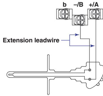
Resistance temperature detector input
