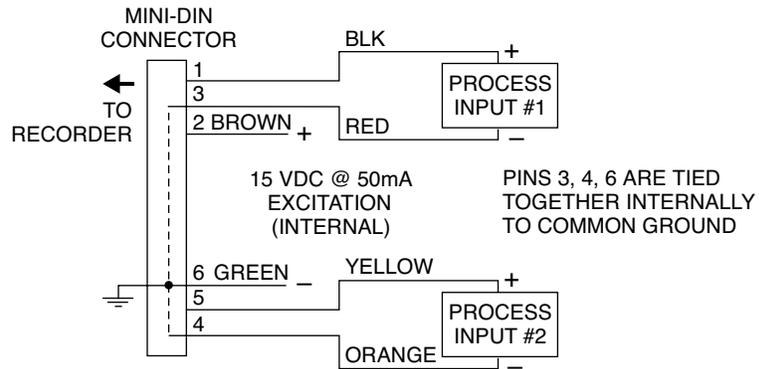
Figure 1-2. Wiring Diagram, Dual Process Input Model, CTXL-DPR
