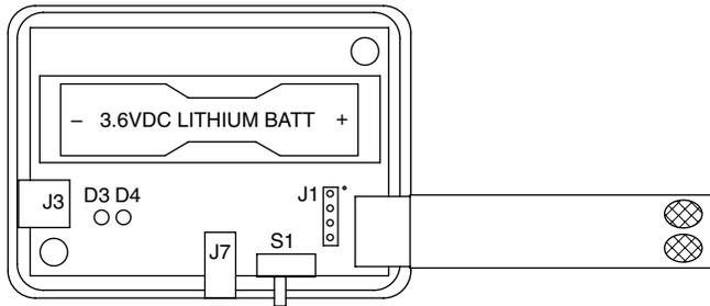
Figure 8-2. Battery Location in the Wireless Transmitter
