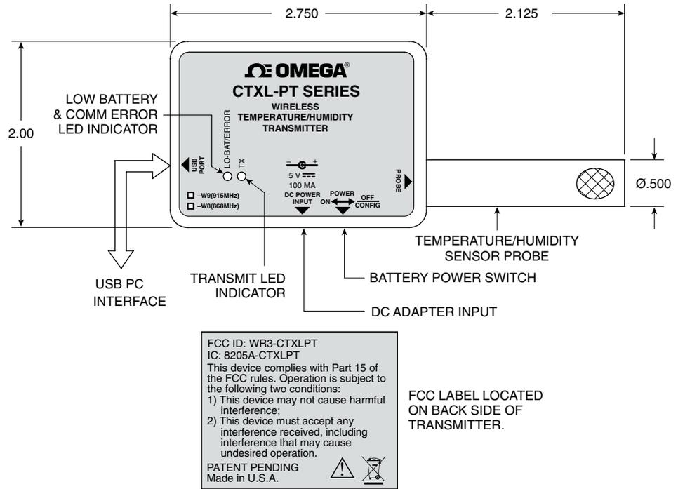
Figure 8-1. Temperature/Humidity Wireless Transmitter, General Dimensions, Labels and Descriptions
