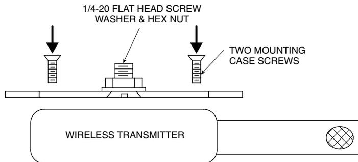
Figure 8-7. Transmitter Mounting Bracket With DIN Rail Mount
