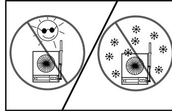
Do not expose the recorder to temperatures other than those stated in the specifications. The recorder can operate in temperatures as high as 120°F (49°C) or as low as 32°F (0°C).
