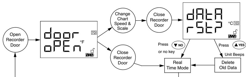
Figure 2-7. Changing Chart Speed and Scale Flow Diagram
