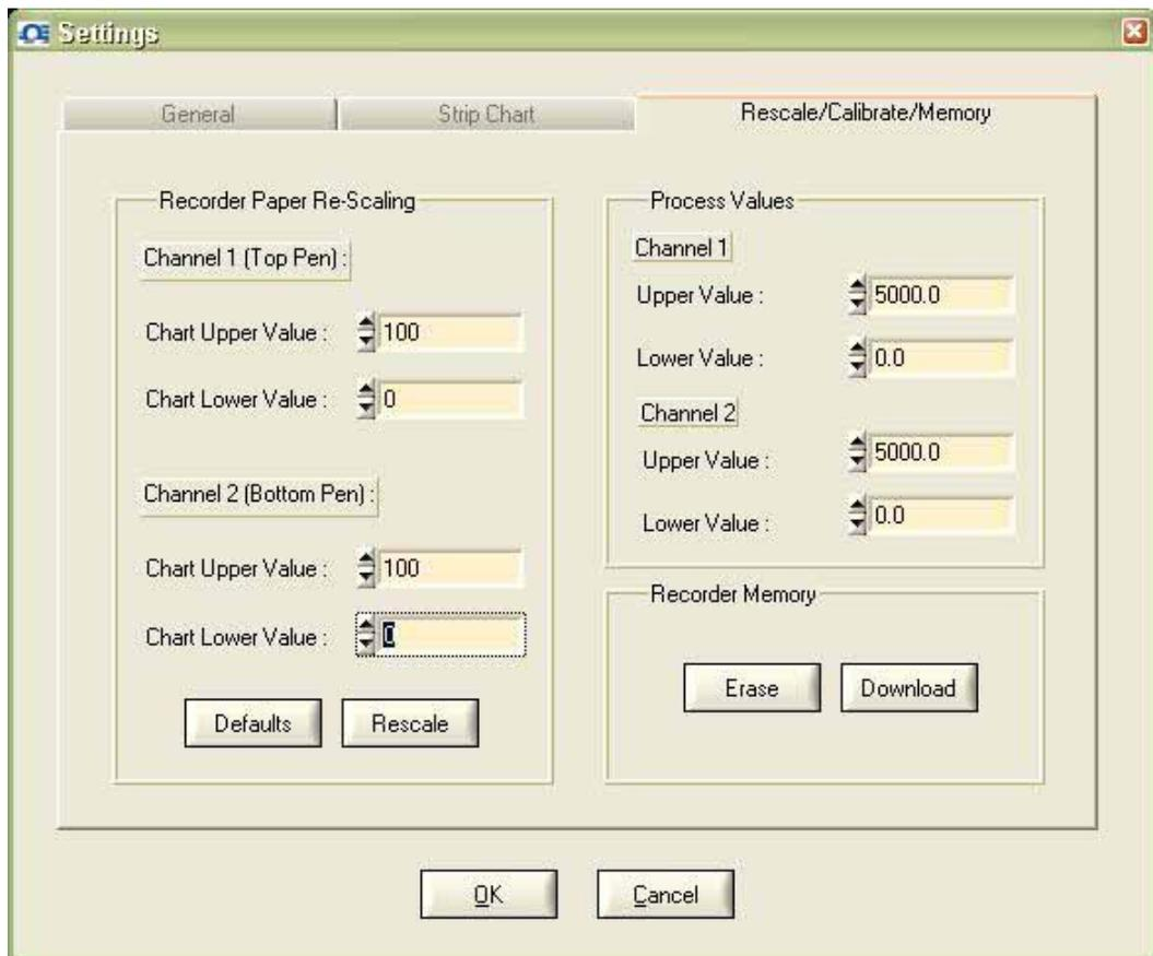
Figure 3-8. Settings Menu - Re-scale/Calibrate/Memory Tab Screen
