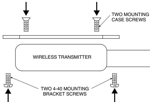
Figure 8-5. Wireless Transmitter Mounting Bracket Assembly
