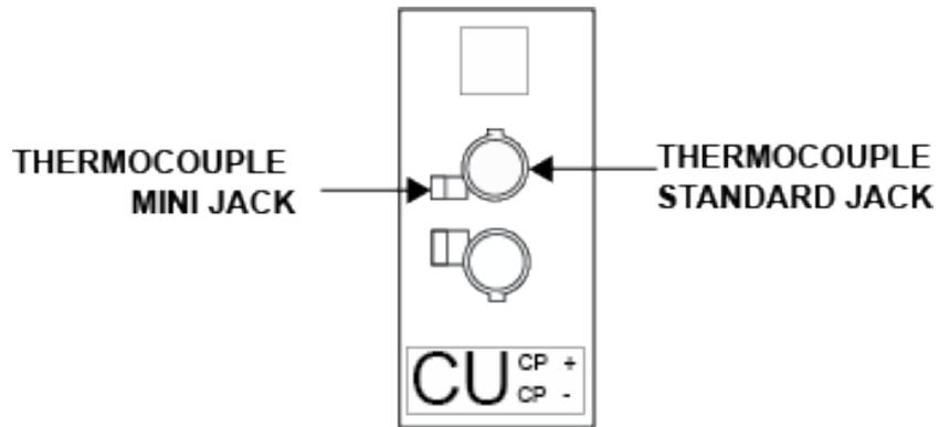
Figure 6. Mini/Standard Thermocouple.
