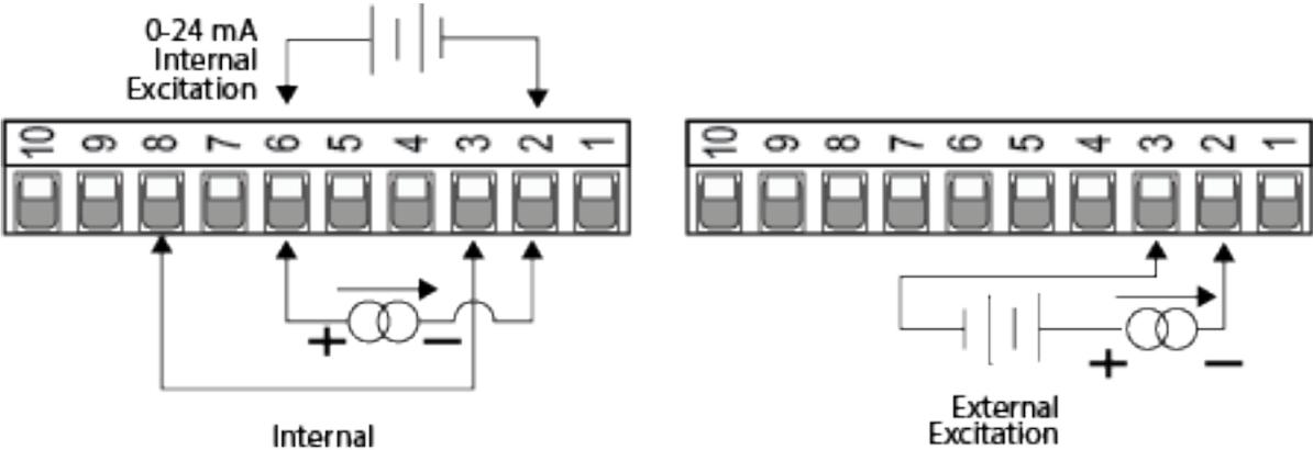
**Figure 5. 4-20 mA Sensor Wiring Diagram.**
