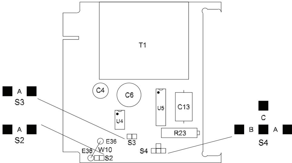
Figure 5.2 Main Board Jumper Locations
