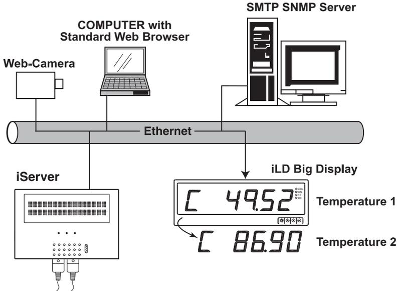
Figure 1.1 iServer and iLD Big Display on the Ethernet Network
