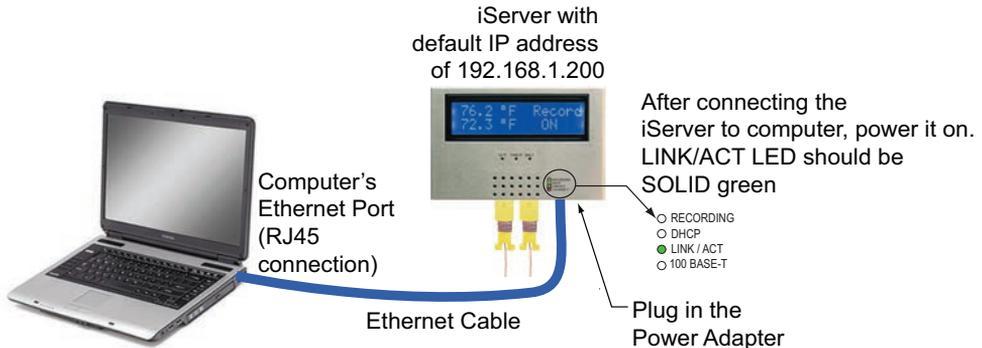
Figure 4.2 Connecting Computer Directly to iServer
