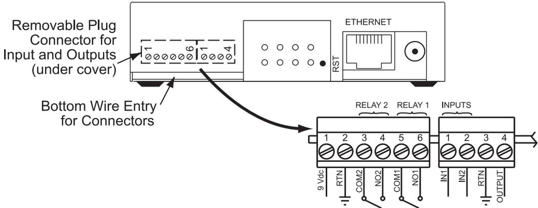
**Figure 2.7 Relay and I/O Contact Connections**
