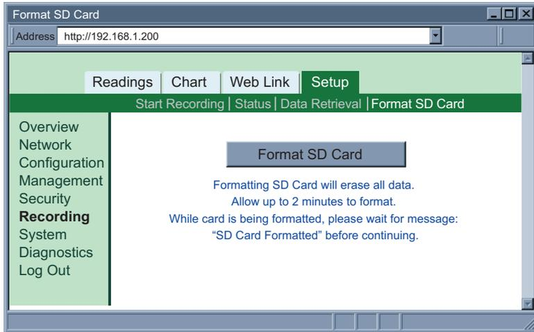
Figure 4.26 Recording Menu: Format SD Card
