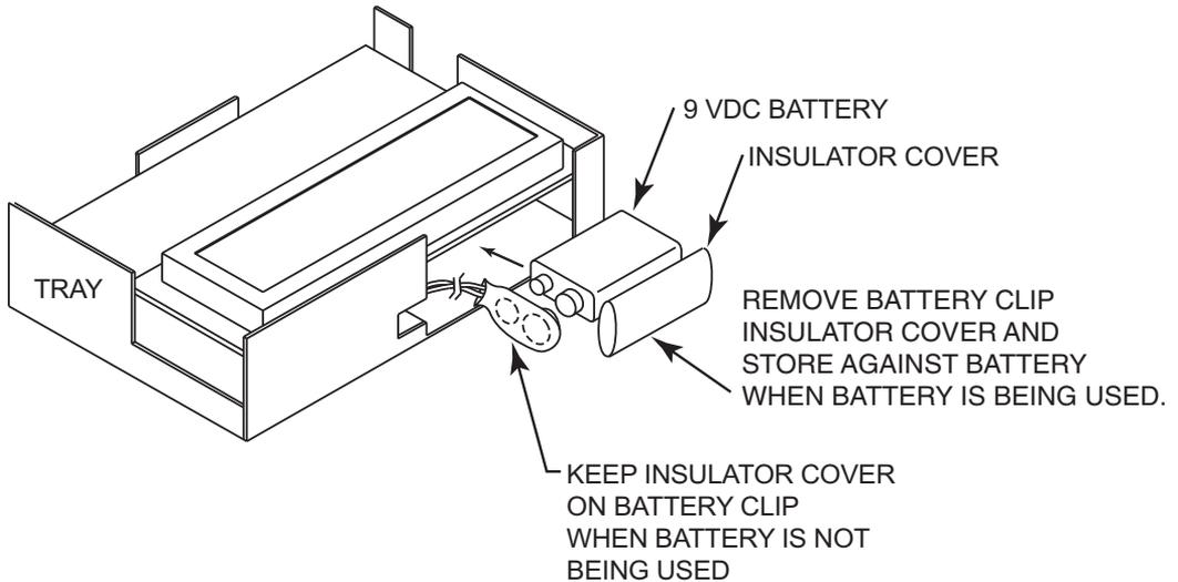
**Figure 2.5 Battery Installation**
