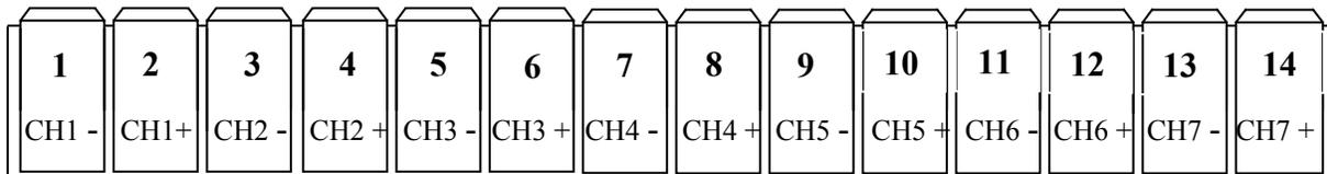
*Table 4. DPS3300 Series Output Connector Pin Assignments*
