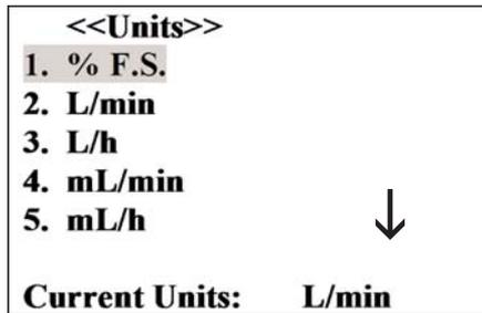
Figure b-4, FMA6600/6700 Units of Measure Screen
