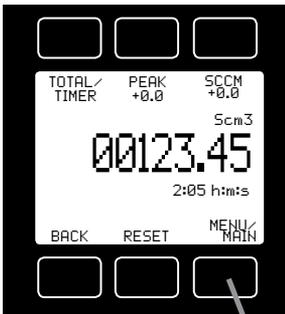
If your meter was ordered with the **Totalizer** option (page 46), pushing the **TOTAL** button once will bring up the **Totalizing Mode** display. Pushing **MENU** will bring up the **Select Menu** display.
