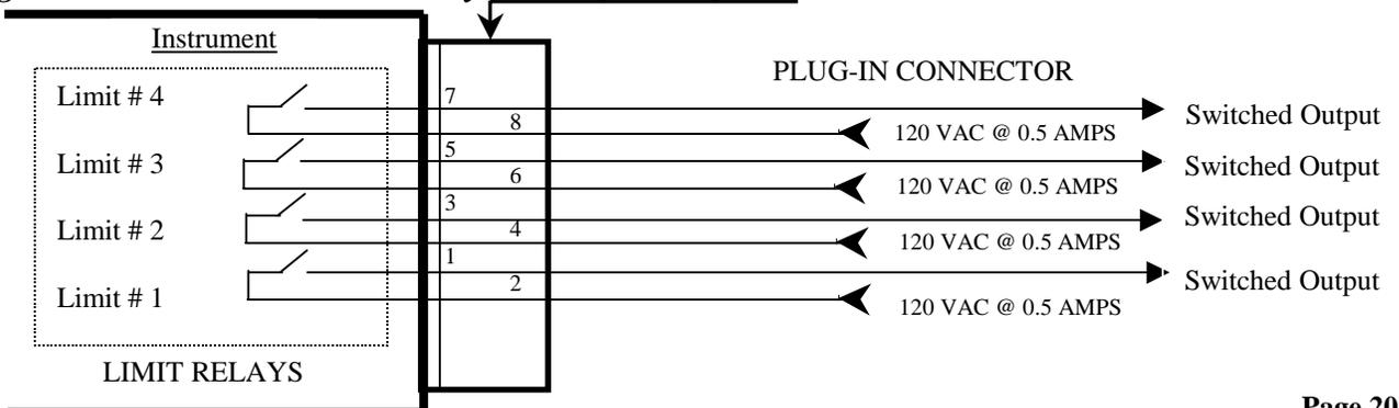
**NOTE: LOOK UNDER SPECIFICATIONS FOR THE RATING ON RELAYS AND OPEN COLLECTOR OUTPUTS. UNDER NO CONDITION SHOULD THE RELAYS AND OPEN COLLECTOR OUTPUTS BE OPERATED BEYOND THEIR RATED CAPACITY. DOING SO CAN DAMAGE THE UNIT PERMANENTLY.**
