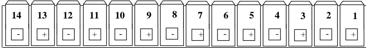
*Table 1. DPS3000 Series Output Connector Pin Assignments*
