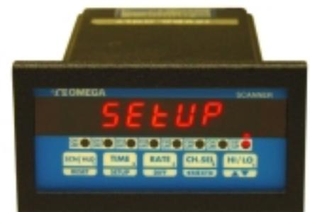
Once the correct pass-code has been entered, the display shows 'SYS CH', with 'CH' blinking. At this point the operator may choose between making channel settings (CH), or system settings (SYS). Use ^v key to toggle between CH and SYS modes. When the desired mode is blinking, press **SETUP** key to begin setup of parameters for that mode. **'SYS' Parameter List**
