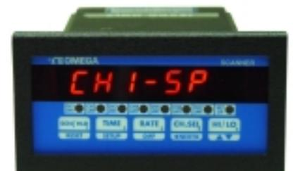
SETPOINT value. Once the desired SETPOINT value is displayed, push **SETUP** key to enter that value and go on to setup channel 1's operational mode.
